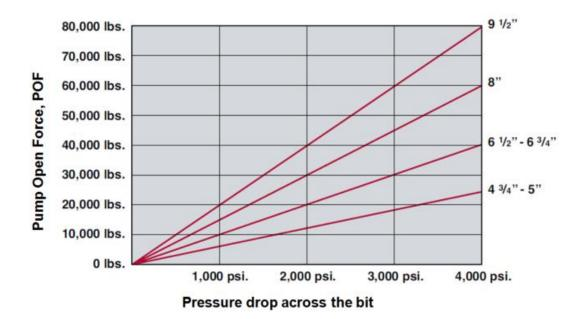
It is recommended to adjust circulation accordingly depending on up/down-jarring and cocking up and down to control the pump open force.
